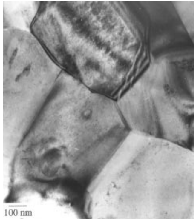
Fig. 6 Transmission electron microscopy micrograph of the material milled for 45 h and hot isostatically pressed after annealing for 3 h at a temperature of ~1300 to 1350 °C. Slight grain growth of the \gamma phase occurred during annealing.
